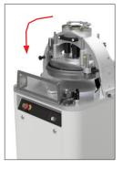
3. Close the cutting unit accompanying it to the support and close the fastening thrusts (x2)
