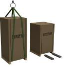
The packaged machine can therefore by lifted with a forklift or pallet truck by inserting the forks in the specific spaces prepared under the packaging. It can also be lifted with a crane, passing the ropes or straps under the packaging. In this case, comply with the maximum tensioning angle of the ropes which must be 45°, as shown in the figure.
