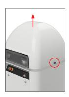
1. Remove the upper casing by unscrewing the specific fastenings (x2)
